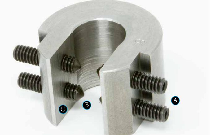
**C** SERRATED SURFACE: Offers increased holding power. **B** CONE POINT: Deep penetration ability, highest tor-sional and axial holding power. A HEX SOCKET: 6 pressure points for ease of driving and strip resistance.
