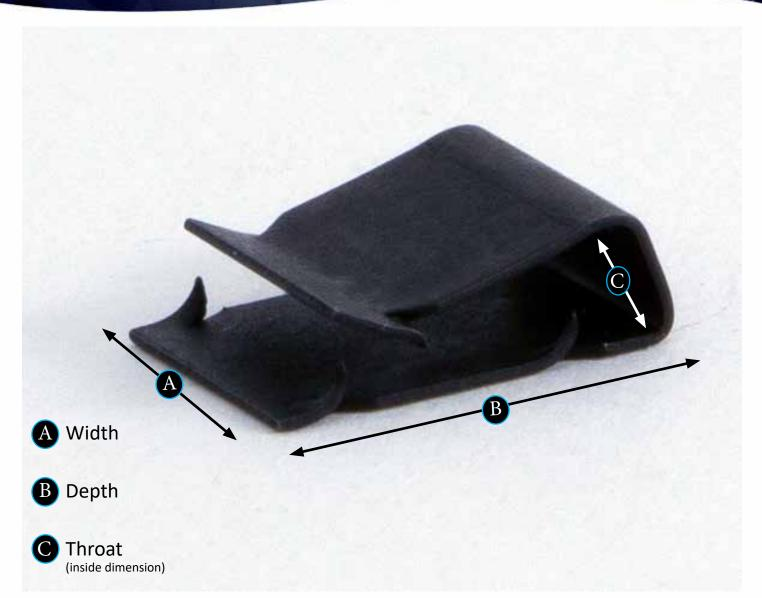
The Extra Wide Black Backward Incline Clip is an answer to our customers' request for a smaller clip with superior gripping power for a thicker fan blade. Perfect for tighter areas where you need a little more weight in a smaller clip, but still need a wider throat to accommodate a thicker blade. Three sets of barbs ensure this clip will stay put even when opened to approximately 3 mm or .125 inches. Available only in black phosphate finish.
